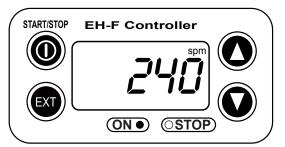
(2) Press EXT key for 3 seconds or more to move to USER mode. The picture below shows the EXT mode selection display.
