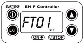
(8) Set a large figure for the long chattering by or key, and set a small figure for high speed (high frequency) chattering. The picture below shows FT04 is selected.
