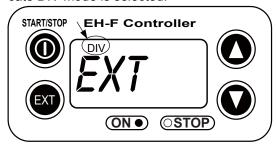
(3) Pushing EXT key, "SET" appears and display shows the mode currently set. Picture below shows ANA. V mode is selected.
