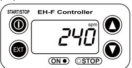
(3) Push EXT key while pump is operating in DIV mode. Pump stop running and "SET" indication appears on the DIV setting display in stead of "spm" indication.
