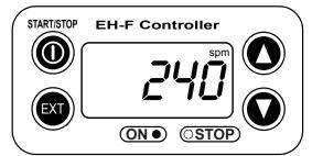
(2) ANA.V indication appears and pump enters an EXT mode as EXT key is pushed once. Pump starts operation in accordance with current signals and various settings. ON lamp blinks at each pumping during operation. Pump is controlled via the EXT mode which was selected at USER mode. The initial setting of EXT mode is ANA. V mode. Select a preferable EXT mode in USER mode. The picture below shows ANA. V mode. (The spm on the display changes according to input signals.)
