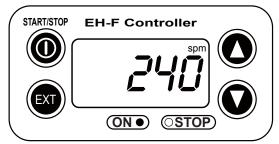
(2) Pushing EXT key, "ANA.R" appears and pump starts running in the ratio of an input pulse signal: pumpings. ON lamp blinks at each pumping. The initial setting of the EXT mode selection is ANA. V mode which is the operation in proportion to current is selected. First select ANA. R mode in USER mode. Refer to P. 40 for more information.
