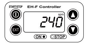
(6) Push EXT key in order to display the current set state. "SET" indication appears. The picture below shows the buffer memory is set to OFF.
