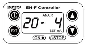
(5) Push EXT key to return to EXT mode. Pump starts to run on the setting at item (4). ON lamp blinks synchronously at each pumping.
