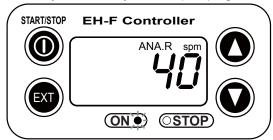
(6) When pushing START/STOP key, pump enters WAIT mode and stops running. ON lamp stops blinking and "ANA.R" disappears.
