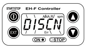
(1) In case Input signals fall to 4 mA or below while 4-20 or 20-4 is set to ANA. R mode, pump stops with "DISCN" blinking and "Err" on display.
