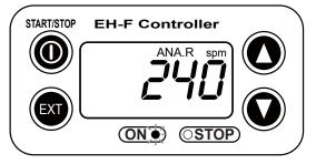
(3) Pushing EXT key when pump is running in the multiply operation calls the setting display of ANA.R mode, and "SET" and "mA" indications appear while "spm" disappears. Pump stops running and ON lamp stops blinking.
