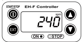
(2) "MULT" indication appears and pump starts running in an EXT operation mode in the ratio of an input pulse signal: pumpings as pressing EXT key. ON lamp blinks at each pumping. Display shows the rest of the number of strokes. In MULT mode the number of strokes is equal to the setting value in manual operation.
