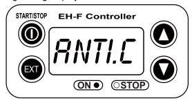
(2) Press EXT key for more than 3 seconds to move to USER mode. The picture below shows pump enters the EXT mode selection.
