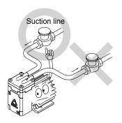
Always use a suction valve to adjust an air/liquid flow.
